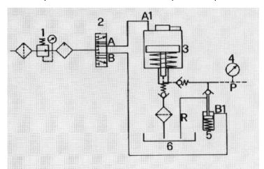
oil pressure is at the highest level. Adjusting the screw inward will hold the valve shut with more force but will also require more pilot air pressure to release it.
